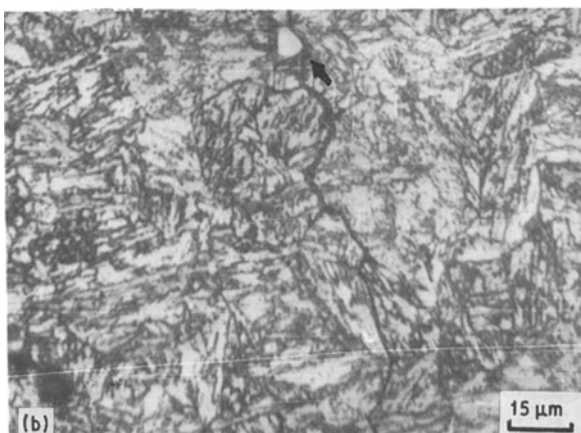
Figure 3 Microstructure at HAZ II/parent metal interface showing (a) crack initiation at a cuboidal inclusion, and (b) crack initiation at an angular inclusion and propagation along the grain boundaries towards parent metal.
