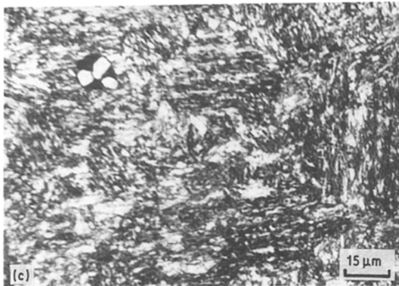
Figure 2 Microstructural features of (a) weldment, (b) light etched HAZ I and (c) dark etched HAZ II.
